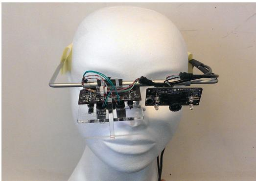
Figure 3: Low-cost head mounted eye tracker
