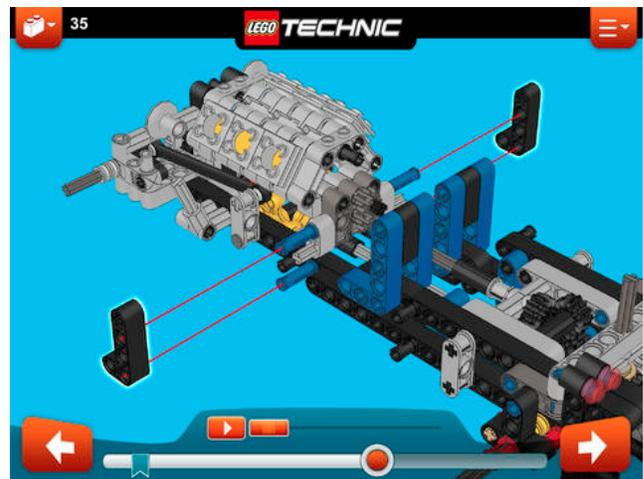
**Figure 1:** LEGO TECHNIC digital building instruction. The slider between the arrows offers forward-rewind; the play button offers a short animation of where to place the two black bricks. Two-finger pinch will zoom and moving the finger on the tablet will rotate the model.
