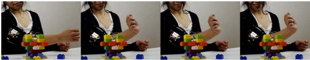
**Figure 3: Experimental scenario: Playing by using muscle activity and LED blocks: She moved her wrist to activate the flexor muscle. Then LED orange color blocks were illuminated.**
