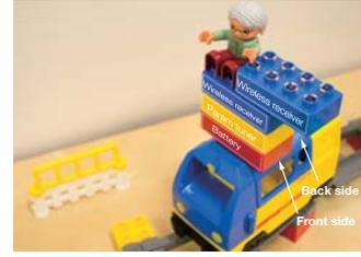
**Figure 4: A developed toy train based on the motor action block**
